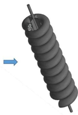
Archimedean screws are mainly used as hydrodynamic screws to drive electrical generators or as screw pumps to convey fluids (as in playground installations).
