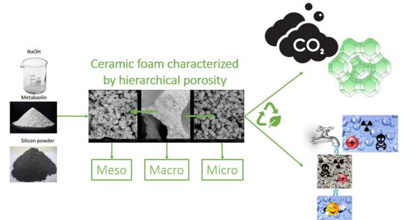
Supporting or shaping zeolites can represent a challenge to obtain this kind of systems. In fact, structuring a porous powder, as a zeolite, permit to obtain an optimized structure with high mass transfer, low pressure drops and high mechanical and chemical stability.
